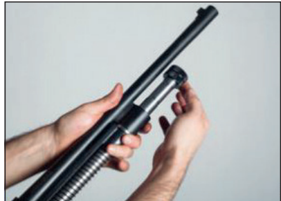
Put the nut on the lower rod and tight it completely.
