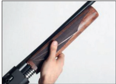
Slide off the foregrip by pushing it forward.
