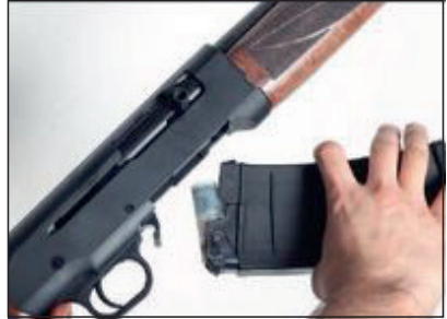
First, insert the magazine from the front side.
