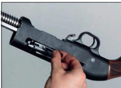
Turn the gun to the opposite direction and place the key pin of the bolt assembly.
