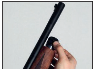
Put the front cape and tight it by moving in clockwise direction.
