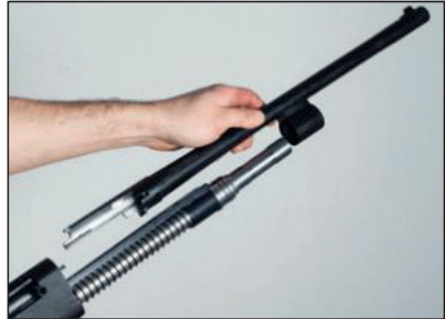
Set the back of the barrel in receiver and also at same time insert to the lower rod too.
