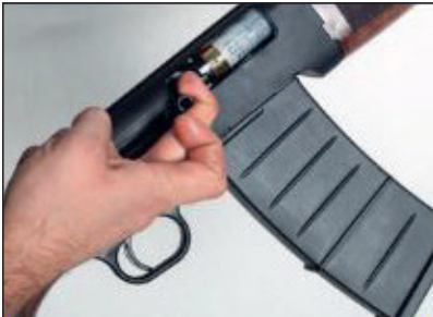
At the end pull back the bolt completely and then leave freely, Gun is ready to fire.
