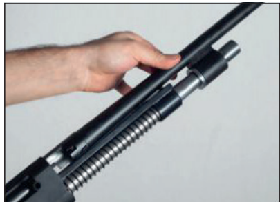
Pull the barrel out.
