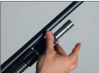
Open the nut by turning in anti-clockwise direction.
