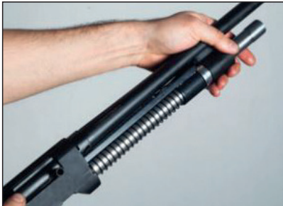
When you are pulling back the barrel at the same time pull back the bolt with your right hand to make the fixation of the barrel.
