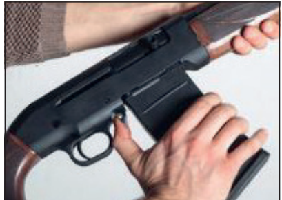
Press the magazine latch to the front side to take off the magazine and pull back the bolt to take off the cartridge which is in the chamber.
