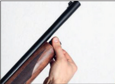
Open the screw from the front side of forend.
