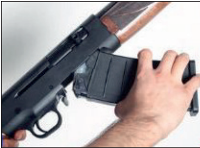
After inserting from the front, now press from the back side of the magazine. Be sure you fixed the magazine completely.
