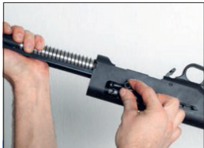
Turn the gun in the opposite direction, press the bolt towards the back like approximately 0.5 cm and take off the bolt key from the left side.
