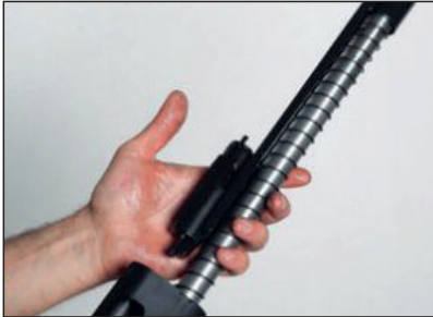
Take off the bolt group with the sliding bar and also with the spring.
